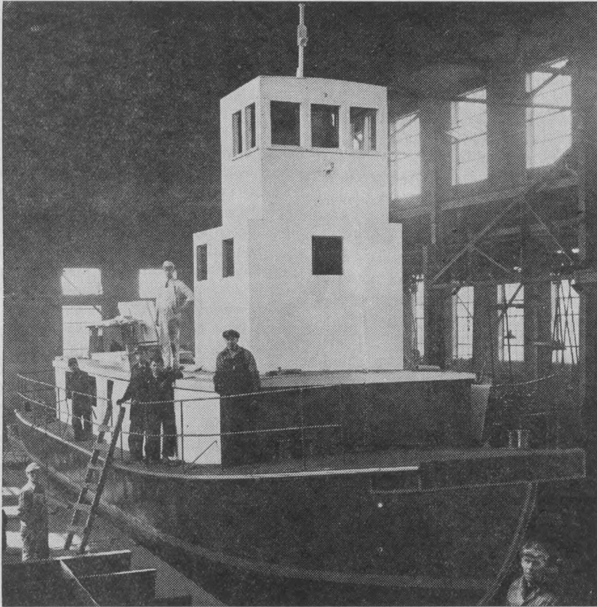
240 H.P. TWIN SCREW DIESEL TUG (during construction) for THE NORTHERN TRANSPORTATION CO. LTD.
